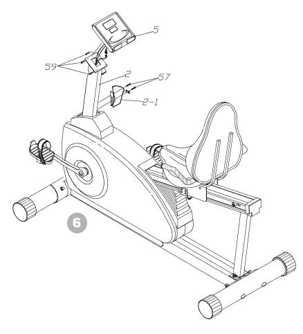
**6.** Connect the computer cable at the top of the console tube (2) to the console (5). Feed the pulse wires from the console (5) down into the console tube (2) and out the rear hole in the handlebar area. Attach the console tube (2) to the console (5) with the screws (59) already attached to back of the console (5). Attach bottle rack to console tube (2).
